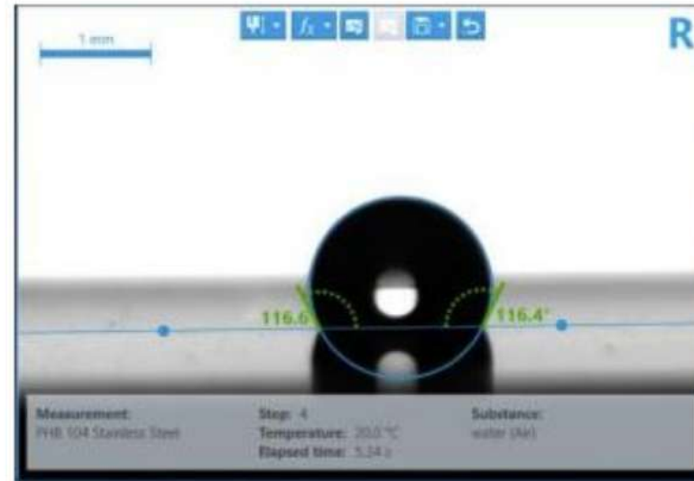
PHB 104 coating on stainless steel
