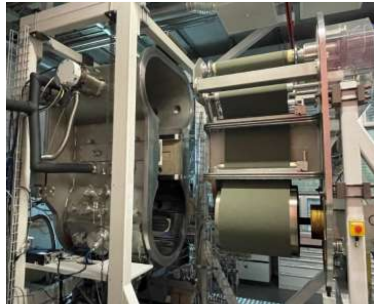
R2R plasma processing (65 cm width)
